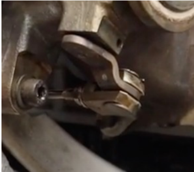
FIGURE 5 2015 VW IS38 TURBOCHARGER LINKAGE ROD END FORK
