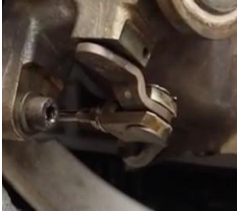
FIGURE 5 2015 VW IS38 TURBOCHARGER LINKAGE ROD END FORK
